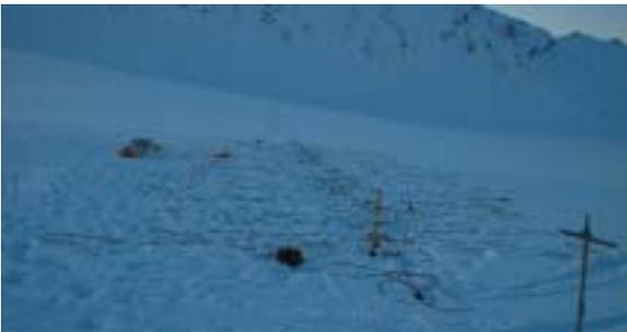
**Above:** Geode seismographs are used to map the subsurface on the island of Svalbard, the most northern community in the world.
