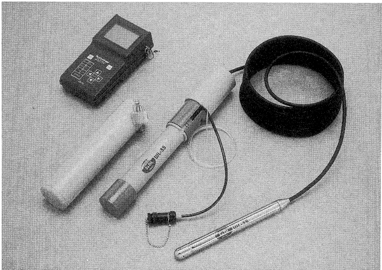
写真-1 SDL水位計の外観 Photo 1 SDL water level meter
