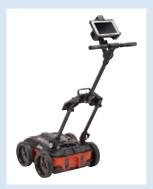
Scanning equipment for underground utility pipes
