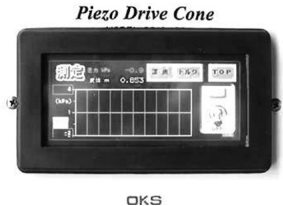
写真-5-2 汎用型PDCの操作パネル Photo. 5-2 Operation panel of universal type PDC
