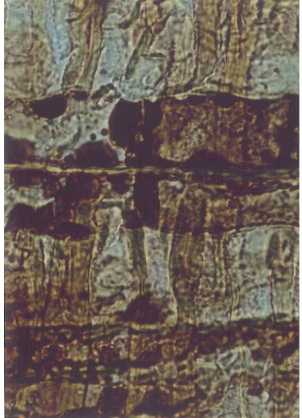
写真 - 6.3 火砕流炭化木放射面切片 Photo 6.3 A radial section of a slice of carbonized wood by the pyroclastic flow
