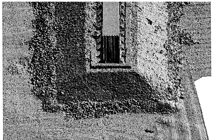
図-8 SeaBat8125で測深した防波堤周辺の海底地形 Fig. 8 A bird's eye view of a breakwater measured with SeaBat8125.
