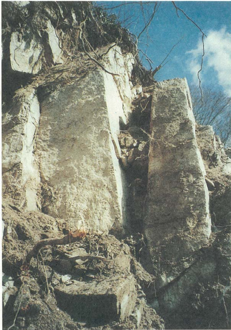
写真-1 斜面舌部付近のトップリング寸前の岩塊 Fig.1 Block just before toppling around tongue of slope.
