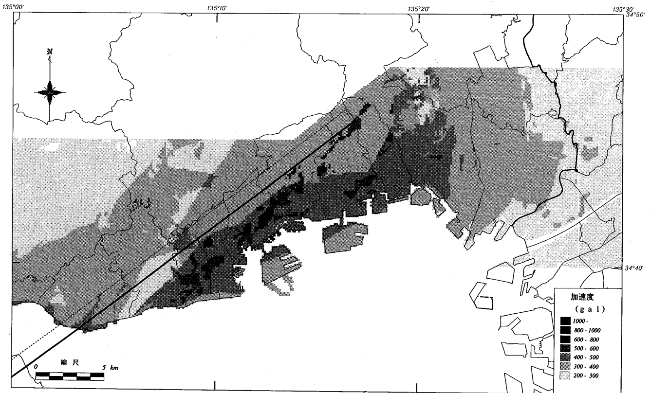
図-7 地表加速度分布 (式(4)による) Fig.7 Surface acceleration distribution (in case of formula (4))
