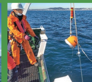
Deepwater microtremor array surveys (jointly developed with Nippon Marine Enterprises, Ltd.)
