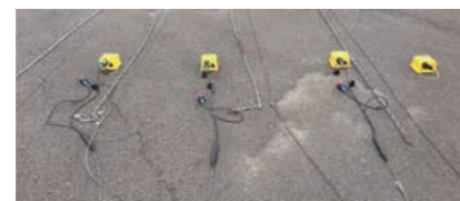
Seabed microtremor array equipment (used in seabed geological surveys for offshore wind power)
