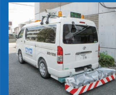
Vehicle used for under-road cavity exploration services
