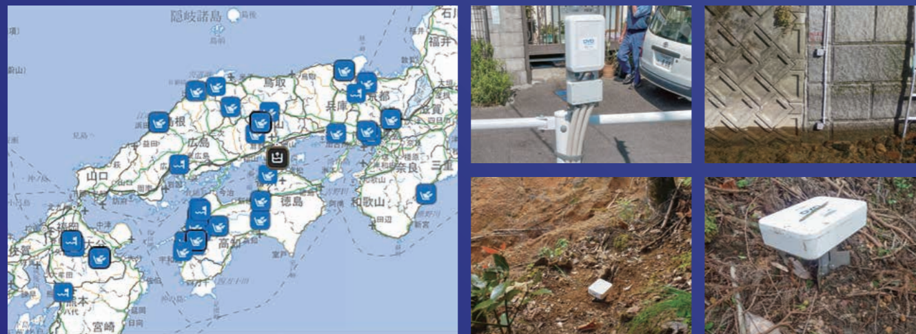
Hazard mapping sensors (flood and slope sensors) and a screen for managing sensor information
