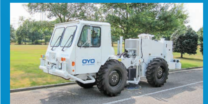
Earthquake simulation vehicle for seismic reflection surveys
