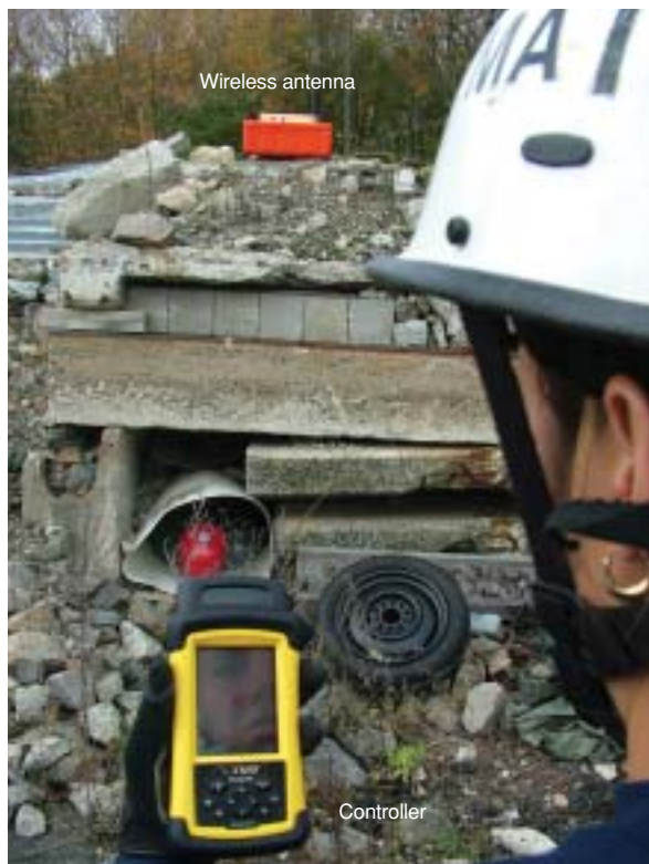
Immediate motion detection, including detection through dense materials such as concrete, brick, snow/ice, mud, etc.
