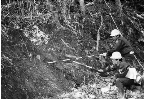
写真-1 尾根部における地形の転倒状況 Photo. 1 Situation of toppling of the stratum in a slope.
