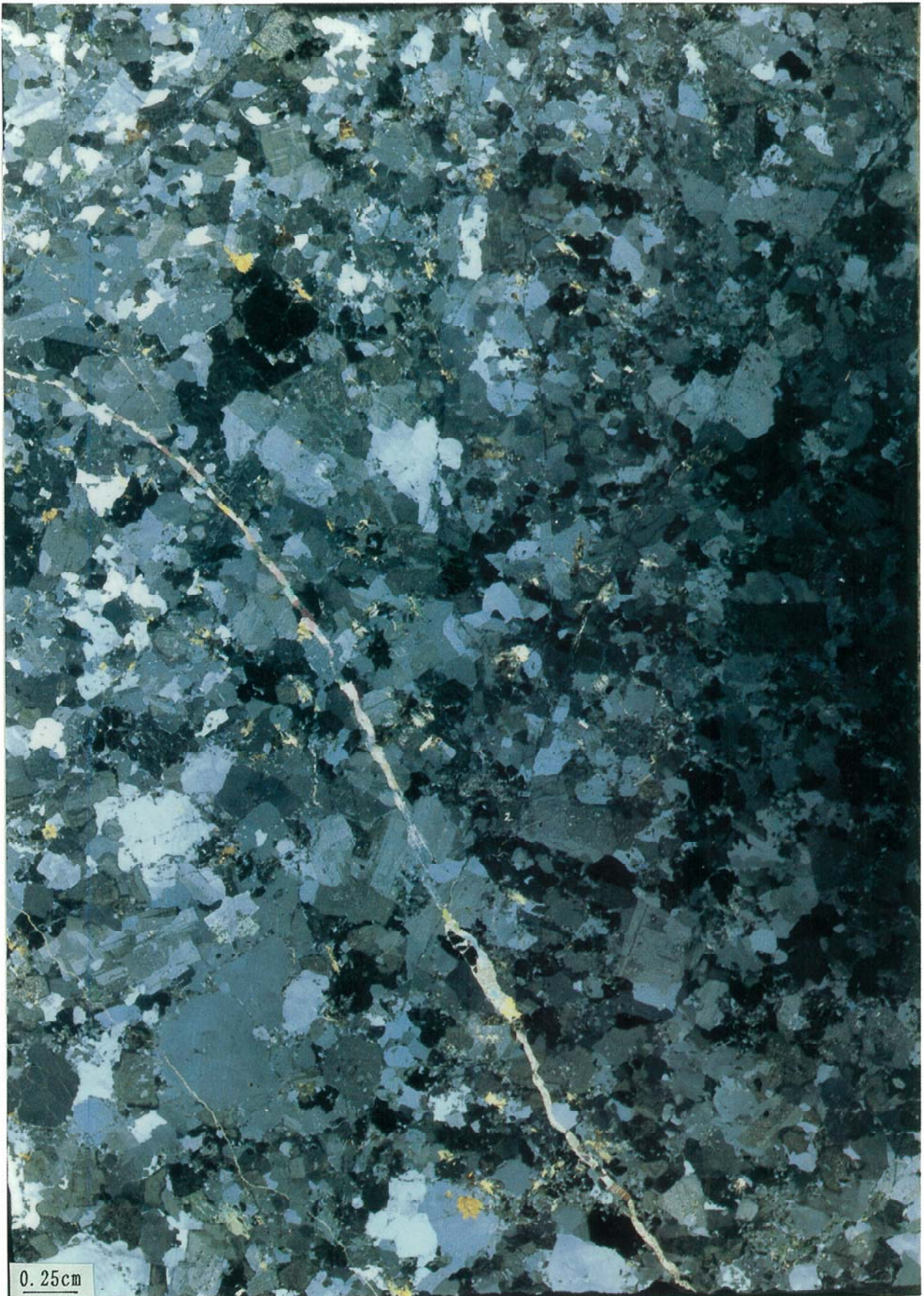
図版-1 718.6m深度の優白質花崗岩コアの顕微鏡写真 Plate-1 Microphotograph of leucogranite core from 718.6m depth.
