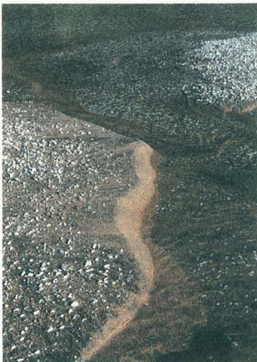
写真-3 放流実験後の流下した方解石 Photo.3 Calcite that moved toward downstream after draw-off experiment
