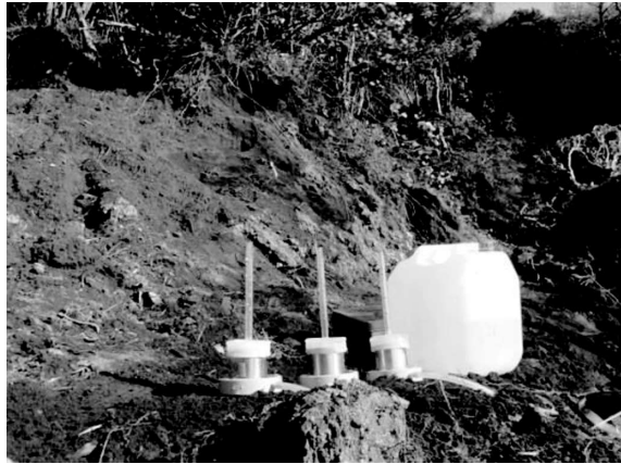
写真-11 簡易透水試験実施状況 Photo 11 Simplified permeability test in progress
